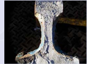
LOF in foot defect
